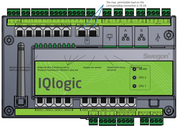
Digital inputs, terminals 4-17, are of extra-low voltage type. Analogue inputs, terminals 18-19 have an input impedance of 66 k $\Omega$ .
