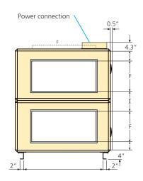
The dimension print shows the connection configuration for fan arrangement 1. For fan arrangement 2 the connections are mirror-inverted. The air handling unit is supplied without end connection panel if a duct accessory housed in an insulated casing will be connected.
