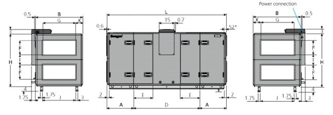
If a water trap (accessory) is fitted, the air handling unit must be raised at least 2 inches to provide space for the water trap. Support feet (accessories) can be used for this purpose. The air handling unit is supplied without end connection panel if a duct accessory housed in an insulated casing will be connected.
