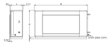
The base frame is always supplied in assembled condition. If the duct accessory is fitted to the upper ductwork, above the duct accessory fitted to the lower ductwork, remove the base beams to the extent necessary, at the building site.
