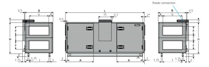
If a water trap (accessory) is fitted, the air handling unit must be raised at least 2 inches to provide space for the water trap. Support feet (accessories) can be used for this purpose. The air handling unit is supplied without end connection panel if a duct accessory housed in an insulated casing will be connected.
