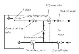
1) The anti-frost protection sensor for the size 05-12 ACLA should be installed in the T-piece on the return pipework and for the size 14-120 ACLA in the connection on the air heater.
