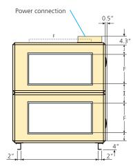
The dimension print shows the connection configuration for fan arrangement 1. For fan arrangement 2 the connections are mirror-inverted. The air handling unit is supplied without end connection panel if a duct accessory housed in an insulated casing will be connected.
