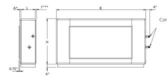
Conn. R male threads. Vents and drain mounted on inlet/outlet connections.
