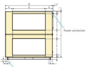
Supplied on 4 inch high support feet. They can be removed or kept as they are when the unit is in place. The unit has provision for fitting the adjustable support feet.
