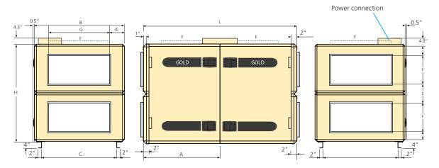
The dimension print shows the connection configuration for fan arrangement 1. For fan arrangement 2 the connections are mirror-inverted. The air handling unit is supplied without end connection panel if a duct accessory housed in an insulated casing will be connected.
