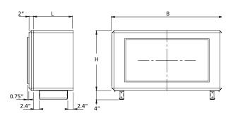
The base frame is always supplied in assembled condition. If the duct accessory is fitted to the upper ductwork, above the duct accessory fitted to the lower ductwork, remove the base beams to the extent necessary, at the building site.
