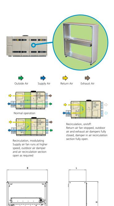
Depending on the version, the damper can be mounted in the upper or lower level
