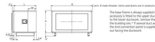
The base frame is always supplied in assembled condition. If the duct accessory is fitted to the upper ductwork, above the duct accessory fitted to the lower ductwork, remove the base beams to the extent necessary, at the building site.\* If several duct accessories are arranged in succession, the end connection panel is supplied only on the duct accessory farthest out facing the ductwork.
