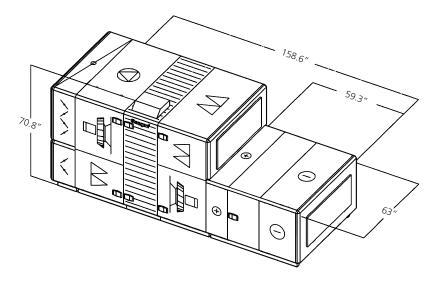
The unit dimensions are shown in the above figure. The approximate weight is 2908 lbs.
