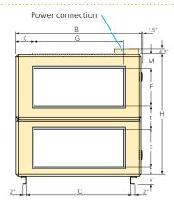
The dimension print shows the connection configuration for fan arrangement 1. For fan arrangement 2 the connections are mirror-inverted. The air handling unit is supplied without end connection panel if a duct accessory housed in an insulated casing will be connected.
