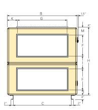
The dimension print shows the connection configuration for fan arrangement 1. For fan arrangement 2 the connections are mirror-inverted. The air handling unit is supplied without end connection panel if a duct accessory housed in an insulated casing will be connected.
