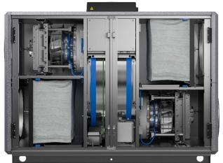
The function of the purging sector requires that the pressure difference is correct and that means, firstly, that the fans need to be correctly positioned so that they are both downstream of the rotor in their respective airstreams and, secondly, that the extract air is correctly throttled to create the correct pressure difference between extract and supply in accordance with our Installation instructions.
