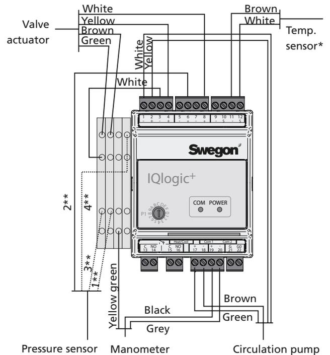
\* Digital temperature sensors require correct polarity when you connect them.
