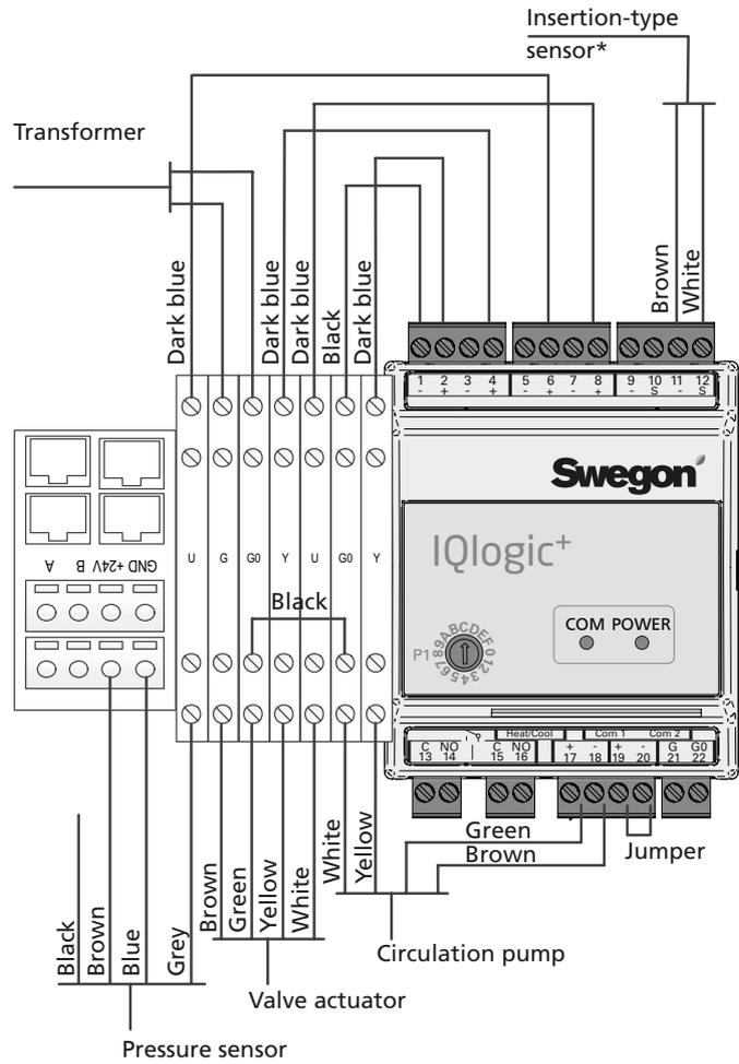
\* Digital temperature sensors require correct polarity when you connect them.
