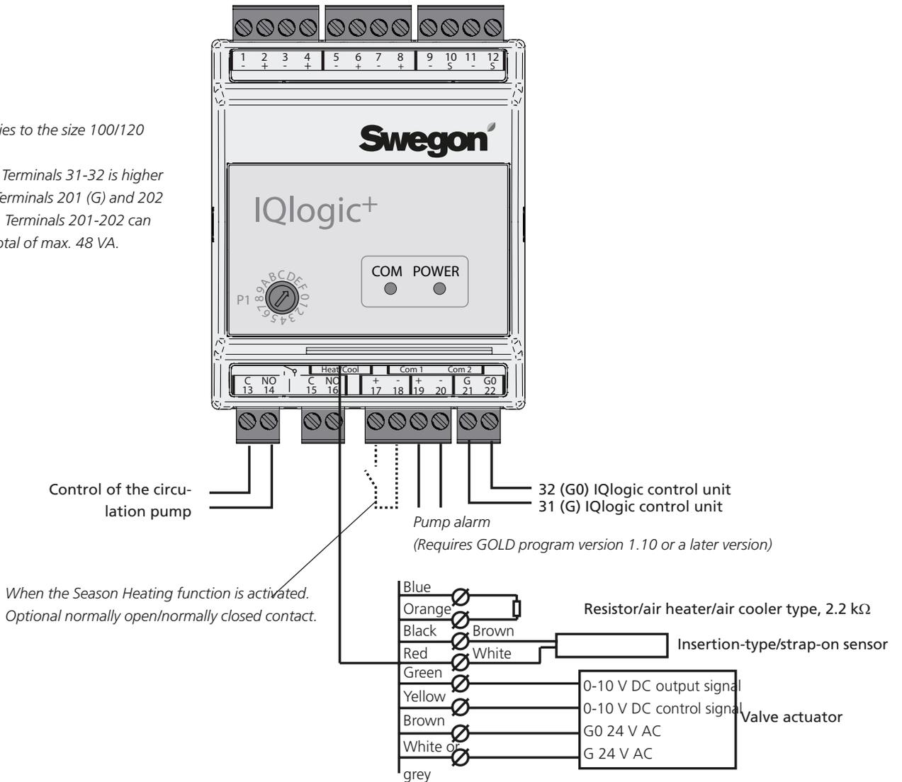
**To wire a standard air heater for the GOLD, TBLE/TCLE**
