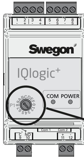
Function selector switch. Position A, B or C.
