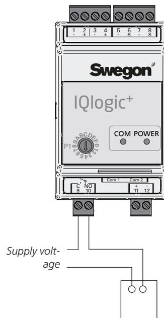
Solenoid valve or circulation pump, evaporative humidifier (not Swegon)
