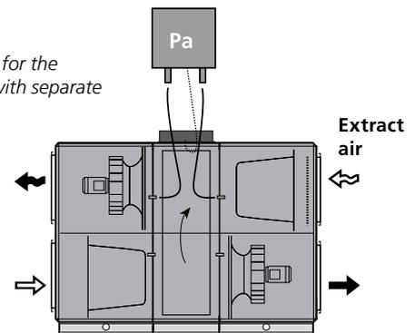
Principle of the Air Quality Control (AQC) function.
