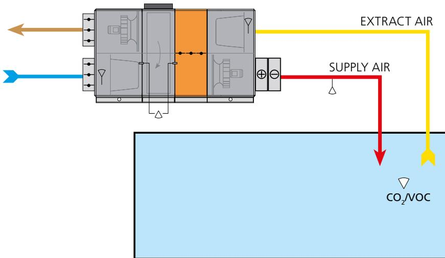
The ReCO<sub>2</sub> function is designed for ensuring the correct air quality or air temperature, by means of recirculating extract air and minimizing the inflow of outdoor air.
