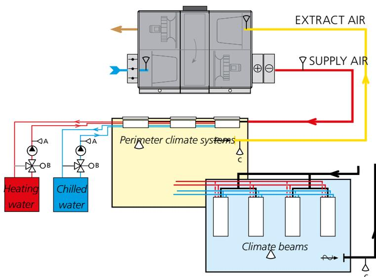
The All Year Comfort function is designed for controlling the primary water circuit for supplying chilled water and/or heated water to climate beams, perimeter climate systems, etc..
