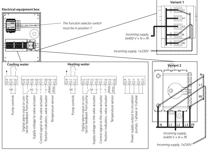
The wiring must be carried out by a qualified electrician in accordance with local electrical safety regulations. The function selector switch must be set to position 7, see the figure above.
