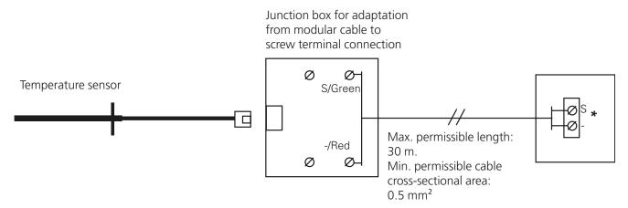
Digital temperature sensors require correct polarity. Be careful when you wire the conductors.
